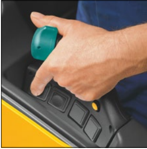
ESE 120: Controls for speed regulation and lift function
