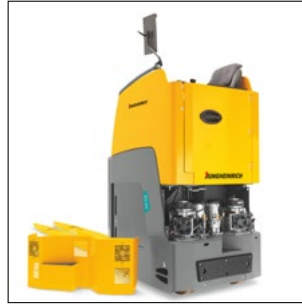
Large service points allow easy access to all main components
