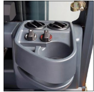
Heating including air demister for windscreen.
