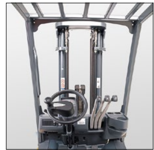
Optimum view of the load thanks to lift mast design giving ideal visibility
