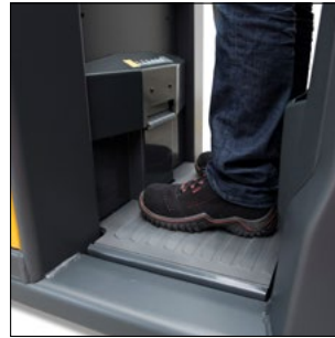
Individually adjustable, sprung comfort stand-on platform (optional)
