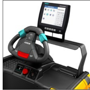
Options bracket with radio data terminal WMT 110 (optional)
