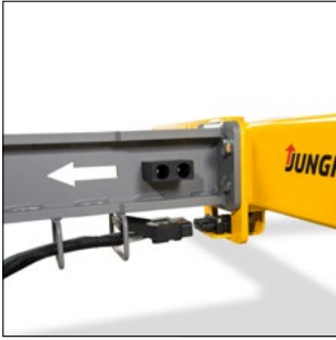
Electrical connection for trailers (GTE 312)
